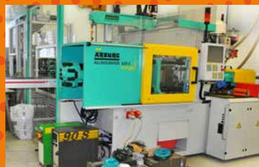
Injection molding machine Arburg Allr. 320C, 5 machines
