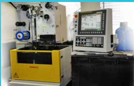
Wire-cut machine Fanuc Robocut - C400iA, 2015
