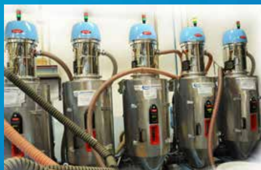
Drying and feeding system Moretto, 2017
