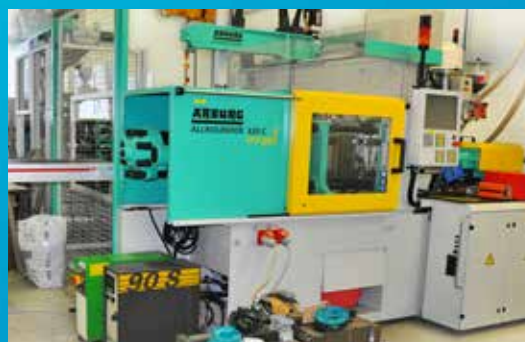
Injection molding machine Arburg Allr. 320C, 5 machines
