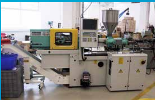
Injection molding machine Arburg Allr. 221K, 5 machines
